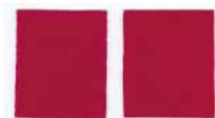
Fabric Before Wash fastness test Fabric After Wash fastness test
