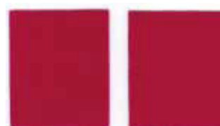
Fabric Before Wash fastness test Fabric After Wash fastness test
